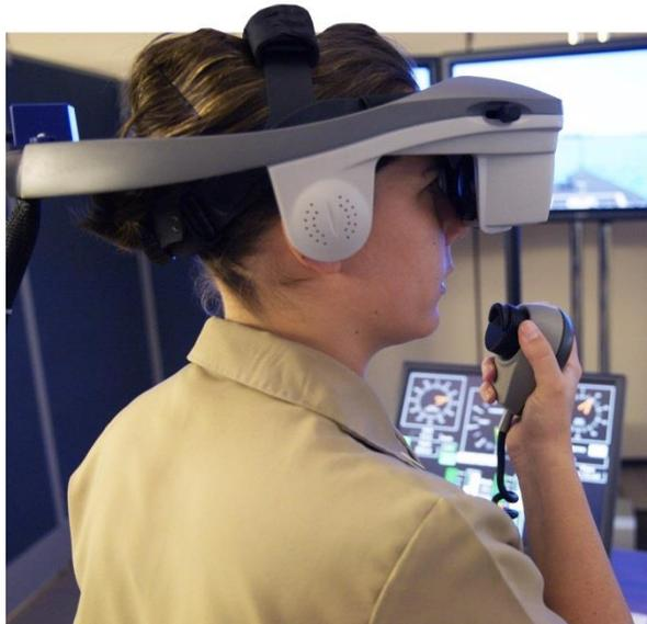
Figure 4 VR Goggles being used for bridge training
